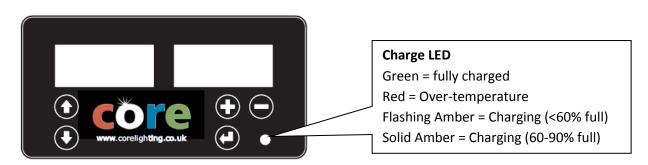
Voltage of the battery can be seen in one of the menu options, achieving full charge at approximately 13.8V (at 20°C). This will fall approximately to 12.5-12.8V once the charger has been removed. The charging current can also be monitored (see DIAGnostics menu 'AN1') and should be around 5 Amps on full-charge, falling when the battery is near capacity.
